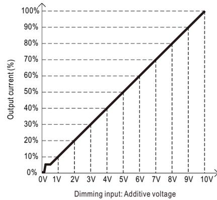
◎ Applying additive 10V PWM signal (frequency range 300Hz~3KHz):
