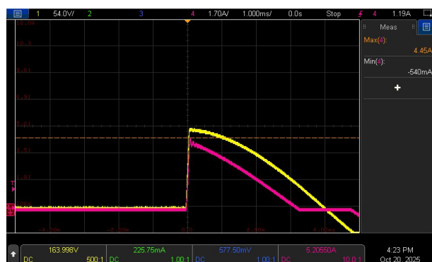
INPUT=115VAC/ 60HZ @ FULL LOAD CH1: AC Input Voltage CH4: Input current
