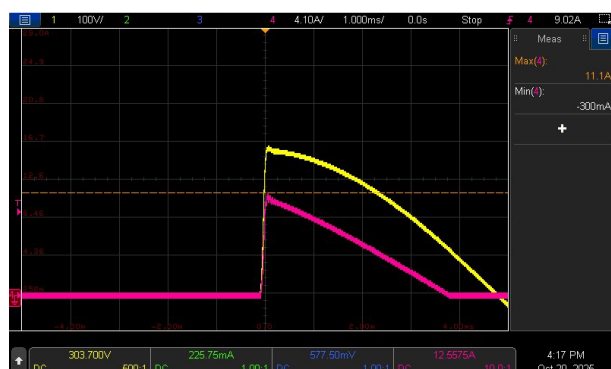
INPUT=115VAC/ 60HZ @ FULL LOAD CH1: AC Input Voltage CH4: Input current
