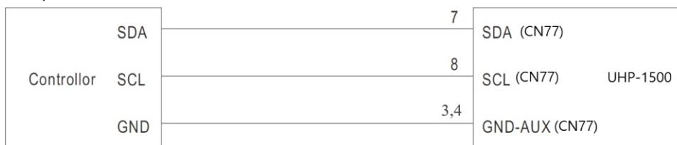
3. Communication function can be accessed immediately after UHP-1500-380 is connected to AC. Set output voltage at 330V.
