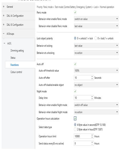
When "Panic mode" is checked, the following parameters appear, which can be used to set the dimming value of the group in panic mode and when the panic mode is released.
