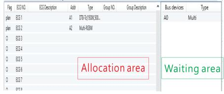
Select the paired lamp and right-click. Not only can you perform on/off and flashing tests online, but you can also modify its DALI short address
