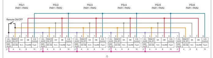
If the lines of PAR1 / PAR2 are too long, they should be twisted in pairs to avoid the noise.
